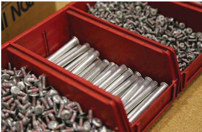
Loctite Dri-Loc threadlocker is applied to the male portion of the threaded rivets before they are shipped to Dee Zee. Photo courtesy Dee Zee Inc.
