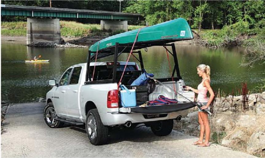
The Invis-A-Rack is a folding cargo rack for pickup trucks. It folds up and locks in place when needed to carry a ladder or canoe. When it's not needed, it collapses into compartments on each side of the bed. Photo courtesy Dee Zee Inc.
